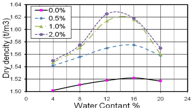
**Fig. 9.** Effect of Addicrete BV on the compaction.
