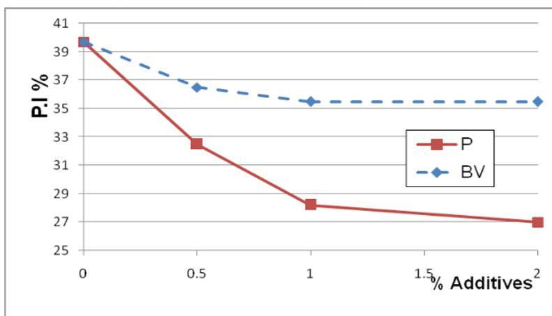
**Fig. 7.** Effect of additives on plasticity index.
