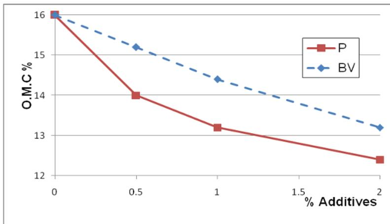
**Fig. 11.** Effect of additives on optimum water content.
