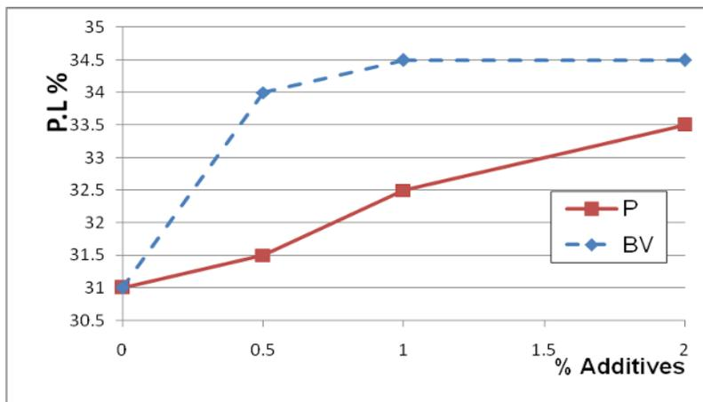
**Fig. 6.** Effect of additives on plastic limit.
