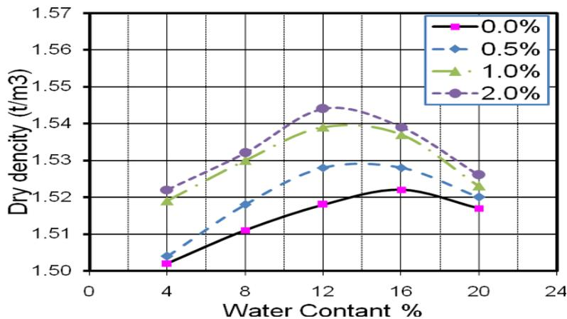
**Fig. 8.** Effect of Addicrete P on the compaction.
